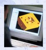
Fixture files are processed in CAD to assign test points, layout of UUT and any special machining. Data is then uploaded to the production equipment for manufacturing.
